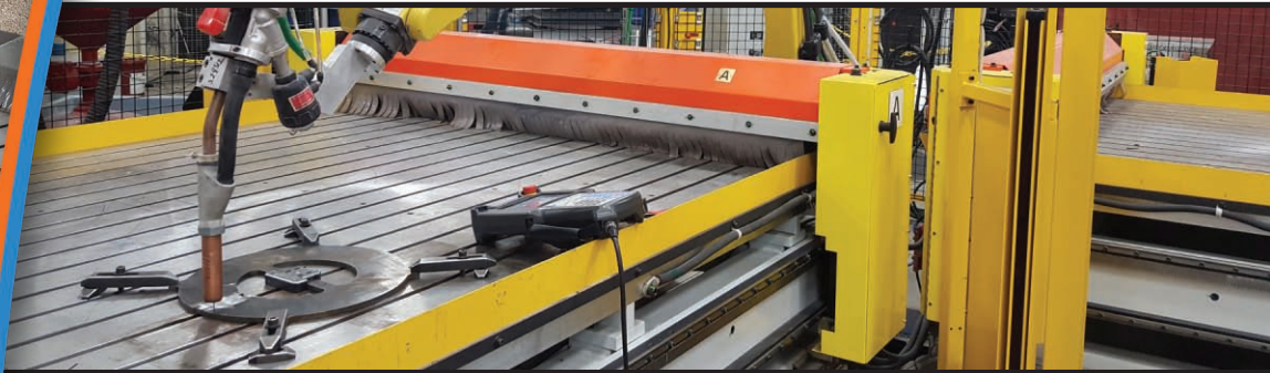
Hard facing auger flighting at Laidig Systems, Inc. in Mishawaka, IN.
